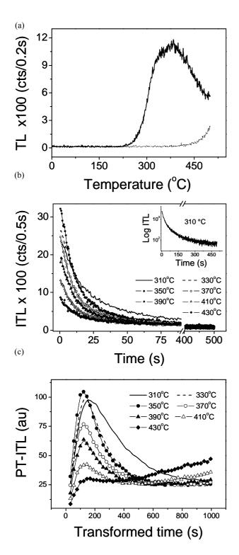
**Figure 3:** a) TL peak of an aliquot of quartz from a modern sample (BTh0) after a dose of 34 Gy and a preheat of 260°C for 10s. TL was measured at the rate of 5°C/s. The dotted curve is the repeat TL run after the TL signal had been measured. b) Natural isothermal TL decay curves measured at different temperatures c) same data plotted as peak transformed isothermal TL (PT-ITL) curves.
