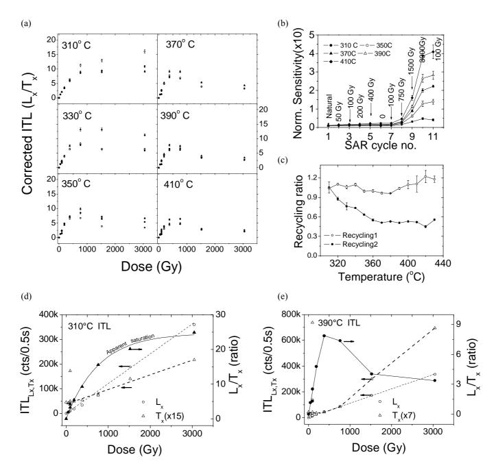
**Figure 4:** a) SAR dose–response curves for some representative ITL measurement temperatures. Three aliquots of the sample K-VII/2B were measured at each temperature. b) Normalised test dose response (with respect to the first value) as a function of SAR cycle or the corresponding regeneration dose (Gy). c) Recycling ratios calculated for the given 100 Gy regeneration doses. Recycling  $I = ITL_{cycle} \sqrt{ITL_{cycle}}$  and Recycling  $I = ITL_{cy$
