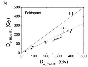
**Figure 9:** a) A comparison of  $D_e$  values derived using ITL at 310°C with those using IRSL from feldspars. Both the signals have been detected using the blue emission. b) A comparison between  $D_e$  values derived using the blue and red ITL signals measured at 310°C.
