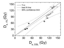
**Figure 6:** Comparison between De values derived using OSL and ITL signal at 320°C from quartz in some young samples.
