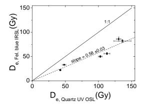
**Figure 2:** A comparison of dose estimates derived using Quartz OSL (UV emission) and Feldspar IRSL (blue emission).
