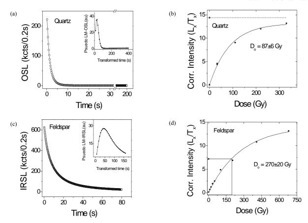
**Figure 1:** a) Natural OSL decay curve from a quartz aliquot of sample K-IX/49. The inset shows a pseudo LM-OSL curve derived from the same data. b) Dose response curve for the same aliquot of quartz. c) Natural IRSL decay curve from a feldspar aliquot of sample K-IX/49. The inset shows a pseudo LM-IRSL curve. d) Dose response curve for the same feldspar aliquot. The first 0.8s was used for signal integration in both IRSL and OSL decay curves.
