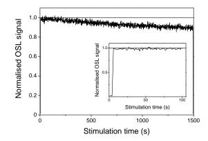
**Figure 2:** Signal observed from an annealed blank silicone-sprayed stainless steel cup during stimulation with blue diodes for 1500 s at 250°C; the signal has been normalised to that observed in the first second of stimulation. The inset shows the signal observed during the first 100 s of stimulation.
