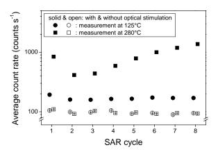
**Figure 3:** Effect of the repeated thermal treatments typical of a SAR protocol on the signals (expressed as average count rates) observed from a blank and silicone-coated stainless steel cup. Stimulation was performed using blue diodes at 125°C and 280°C (circles and squares, respectively); the open symbols indicate the signals observed without optical stimulation. The aliquot was not beta irradiated during the course of this experiment.
