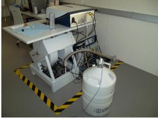
**Figure 1:** CENIEH's ESR spectrometry area: EMXmicro 6/1 Bruker ESR spectrometer connected to an ER4141VT Digital Temperature control system (with the flexible metal transfer line option).
