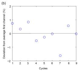
**Figure 2:** (a) Decay curves for one empty stainless steel cup during the first four seconds of OSL (125°C, 40 s) for nine measurement cycles including irradiation (30 Gy), pre-heat (200°C, 10 s), and IRSL (60°C, 100 s) prior to OSL stimulation. (b) Deviation in percent from average signal in first channel for the nine measurement cycles. The line at 0 along the y-axis represents the average signal.
