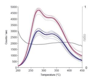
**Figure 7:** TL glow-curves of sample 5 (Devonian siltstone). Upper curves (thick line: mean) NTL after  $150^{\circ}$ C preheat for 19 h only (T). Lower curves: (thick line: mean) NTL after  $150^{\circ}$ C preheat for 19 h and simultaneous 1 GPa pressure (P+T). Grey line: ratio of (P+T)/T.
